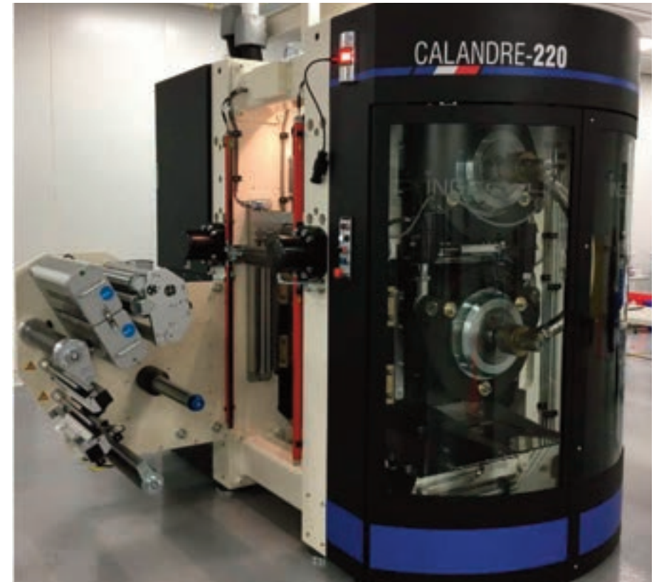
Figure 16 - Teknek cleaning machine with calendaring equipment
