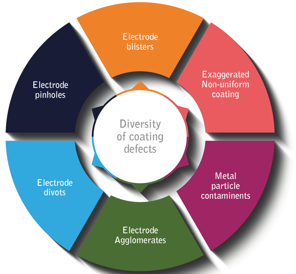
Figure 12 - Types of coating defects
